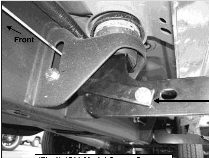
(Fig 6) 1500 Model Center Support Bracket Installation Pictured
